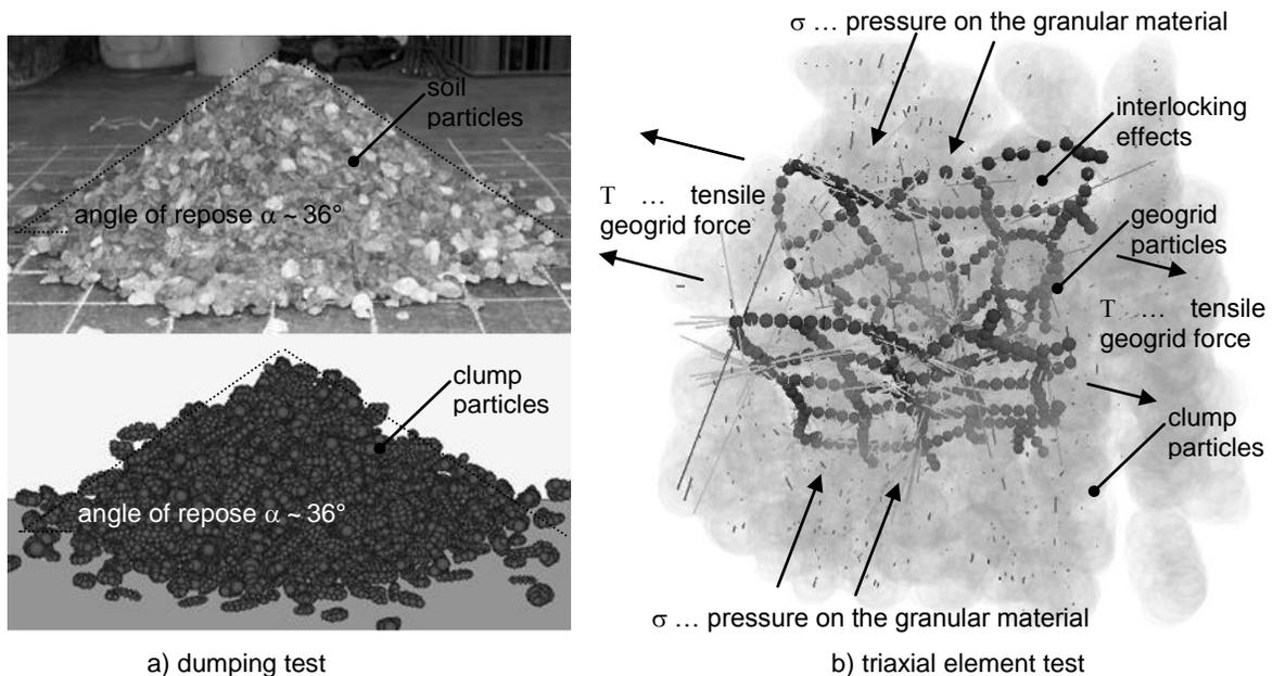
First soil and geogrid have to be calibrated separately. For example the granular particle friction coefficient  $\mu$  can be numerically defined by performing dumping tests (Figure 5a). Missing parameters should finally be calibrated by tests in which the geogrid reinforcement and the granular coarse grain soil material interact (e.g. triaxial tests, Figure 5b).
