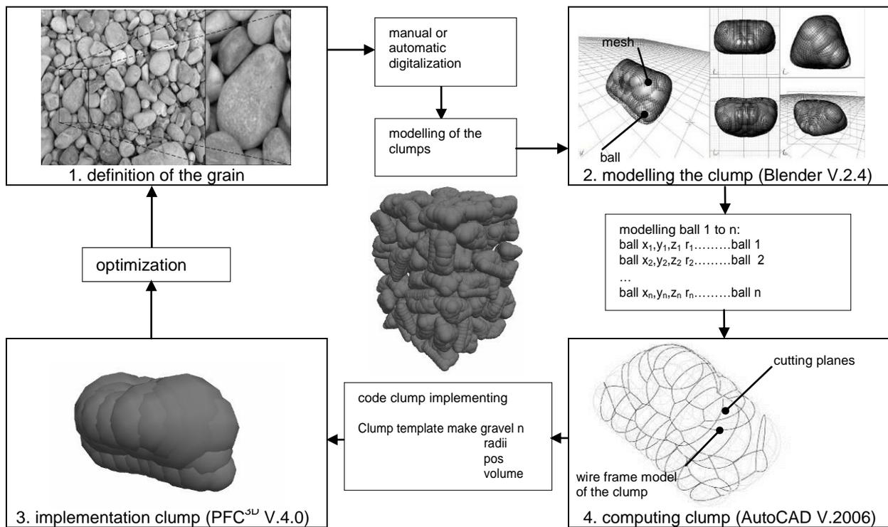
In order to describe the granular experimental material by discrete modelling the 4 typical grain shapes (chapter 3.2) have been selected to categorize and consecutively model the shape of the grains numerically by clumps.
