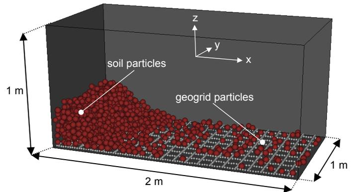
Figure 2. Generated model with the Particle Flow Code.
