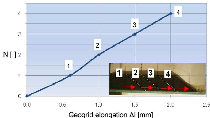
Figure 7. Geogrids elongation after filling and compacting with the compaction advice (Chapter 2)
