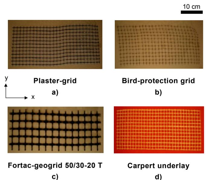
Figure 4. Soft material validation for small scale labtest.
